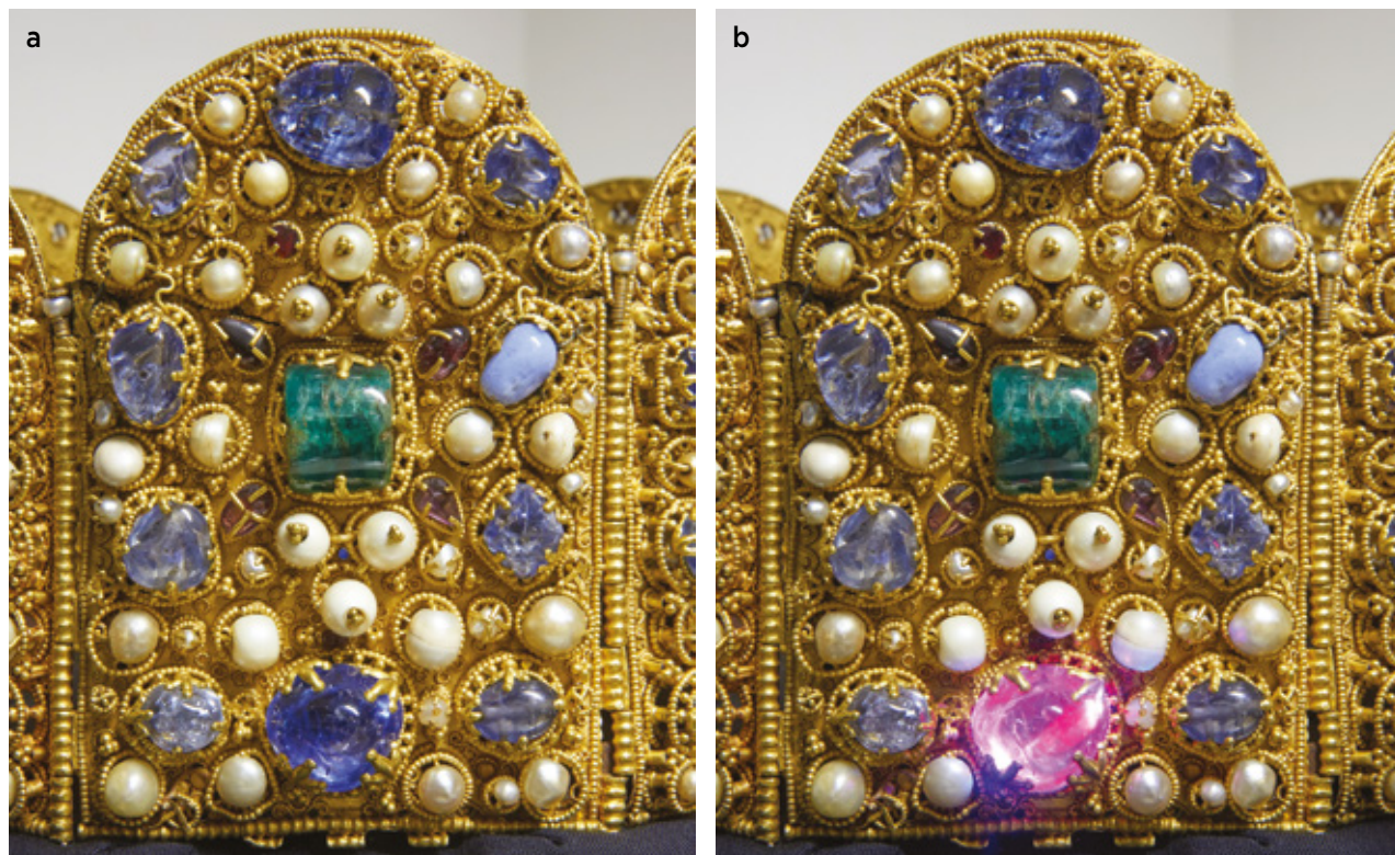
Figure 9: A large, transparent sapphire in the bottom centre of the circlet's right temporal plate (stone G62; 2.1 cm long) shows (a) vivid blue colour in ambient room lighting, but (b) intense pinkish red emission from a 407 nm laser pointer. Photos © KHM-Museumsverband (Christian Mendez); reproduced with permission.
